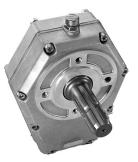
Group 2 pump, splines coupling with 18 splines, tightening torque nut 32-35 Nm. Group 3 pump, splines coupling with 18 splines, tightening torque nut 50-55 Nm.
