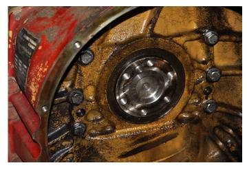
Ensure that there is no leakage around the crankshaft.
