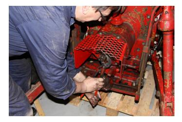
Make sure that the splines on the gearbox's input pin and the power take-off's drive slide easily in position on the clutch. Do not force the tractor halves with the bolts! Damage during installation is not covered by the warranty. The position of the power take-off's position is adjusted here when the power take-off is in the engaged position (independent position). This applies to mechanical power take-offs.
