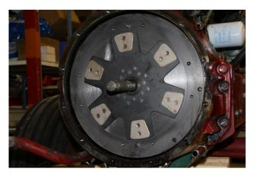
Make sure to centre the plate when assembling the clutch.
