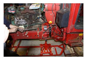
Exercise care to ensure the tractor's both halves are centred in height and laterally when assembling. If this is not the case, installation damage can occur the plate and clutch.
