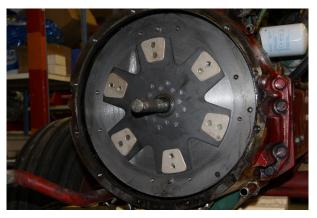
Make sure to centre the plate when assembling the clutch. Use a mandrel intended for this purpose.
