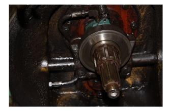
Check the release bearing mechanism with regard to wear and damage.
