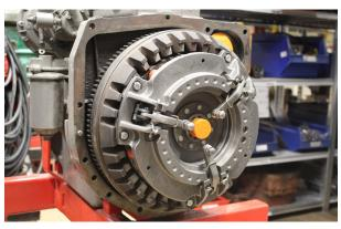
In the case of a double clutch, both the plates must be in the centre.
