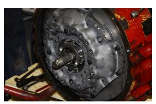
Do not forget to remove the transport locks when dismantling the clutch.
