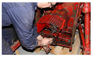
Make sure that the splines on the gearbox's input pin and the power take-off's drive slide easily in position on the clutch. Do not force the tractor halves with the bolts! Damage during installation is not covered by the warranty. The position of the power take-off's position is adjusted here when the power take-off is in the engaged position (independent position). This applies to mechanical power take-offs.
