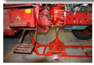
Before the tractor is opened: Make sure that the tractor is jacked firmly and that the tractor can be adjusted vertically during reassembly.
