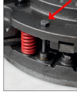
Different types of transport locks. Make sure that the transport locks have been removed before assembling the tractor!
