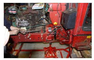
Exercise care to ensure the tractor's both halves are centred in height and laterally when assembling. If this is not the case, installation damage can occur the plate and clutch.
