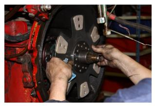
Check that the new plate slides easily on the pin's splines.
