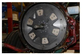
Make sure to centre the plate when assembling the clutch. Use a mandrel intended for this purpose.
