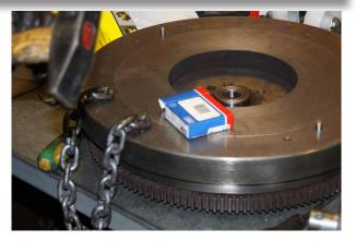
After dismantling the flywheel **must** be machined according to the manufacturer's instructions. Fit a new flywheel bearing.
