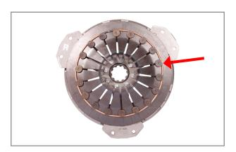
NOTE! This is NOT a transport lock and must not be dismantled.
