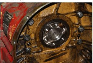
Ensure that there is no leakage around the crankshaft. If there any leaking oil, the crankshaft seal needs to be replaced.
