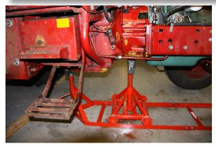
Before the tractor is opened: Make sure that the tractor is jacked firmly and that the tractor can be adjusted vertically during reassembly.
