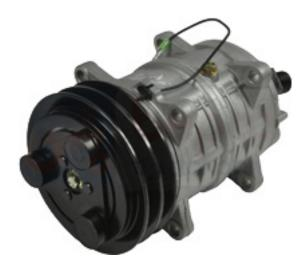
The compressors we sell are supplied with a small quantity of delivery oil that needs to be drained and replaced with the right type and quantity according to the vehicle manufacturer's recommendations.
