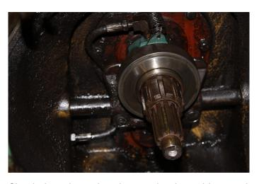
Check the release bearing mechanism with regard to wear and damage.
