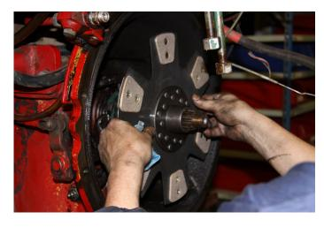
Check that the new plate slides easily on the pin's splines.
