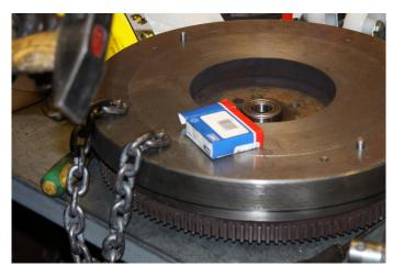
After dismantling the flywheel **must** be machined according to the manufacturer's instructions. Fit a new flywheel bearing.
