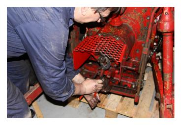
Make sure that the splines on the gearbox's input pin and the power take-off's drive slide easily in position on the clutch. Do not force the tractor halves with the bolts! Damage during installation is not covered by the warranty. The position of the PTO shaft is adjusted here when the power take-off is in the engaged position (independent position). This applies to mechanical power take-offs.
