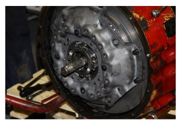
Do not forget to remove the transport locks when dismantling the clutch.
