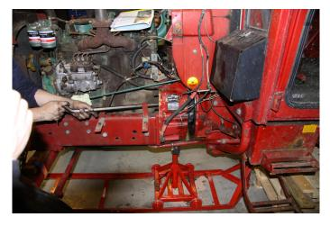
Exercise care to ensure the tractor's both halves are centred in height and laterally when assembling. If this is not the case, installation damage can occur the plate and clutch.
