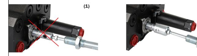
The wire must not be connected directly to the valve coil (figure 1) without first screwing in the sleeve and then connected to the valve coil (figure 2)
